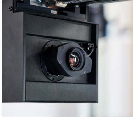
Camera system based on a CMOS sensor
